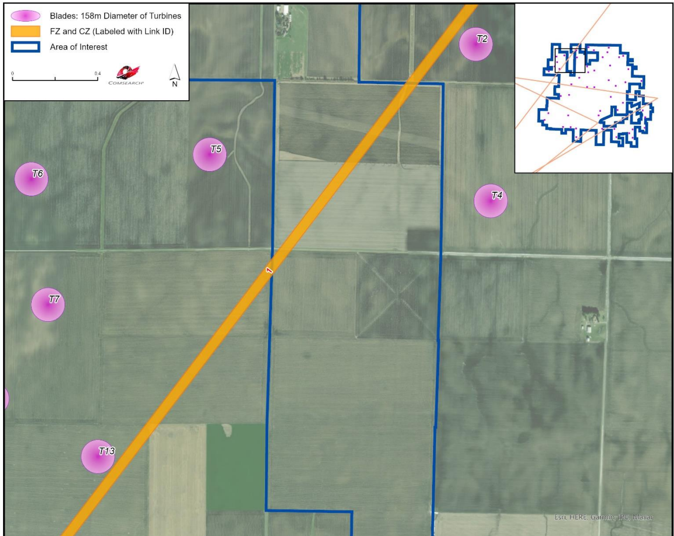
Figure 4: Microwave Paths with Fresnel Zones (North)
