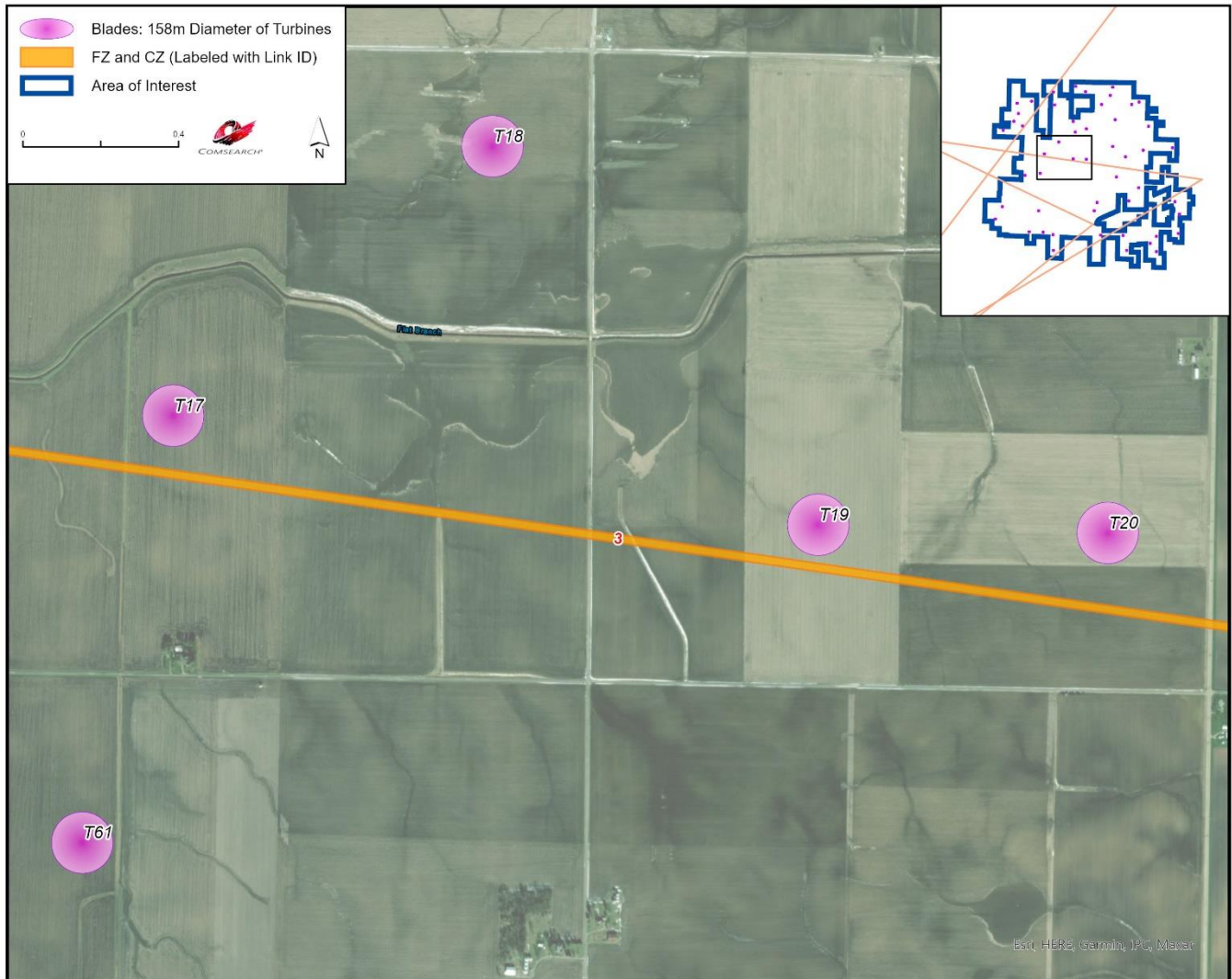
Figure 5: Microwave Paths with Fresnel Zones (Center)
